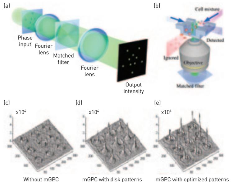
(a) An mGPC is used to generate intense light for particle sorting. (b) Intensity profiles are generated using two LCoS pico-projectors as binary phase input and matched phase filter: (c) without the filter, (d) using phase disks as the input phase pattern and (e) using an optimized binary input phase and matched filter.
