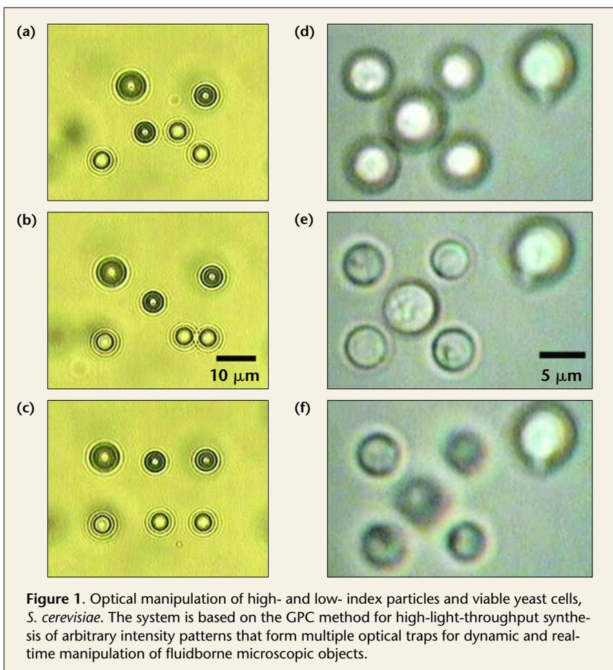
**Figure 1.** Optical manipulation of high- and low-index particles and viable yeast cells, *S. cerevisiae*. The system is based on the GPC method for high-light-throughput synthesis of arbitrary intensity patterns that form multiple optical traps for dynamic and real-time manipulation of fluidborne microscopic objects.
